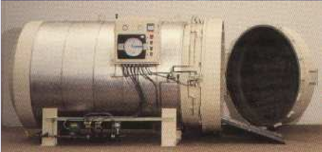
Autoclave With Safety Interlocks on the Door
